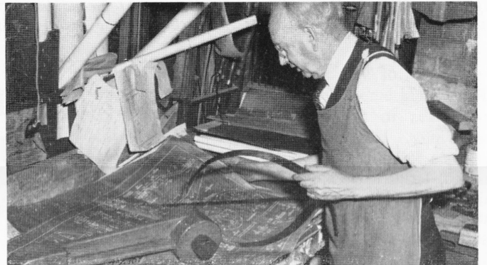
Once a wooden part is completed, it's checked against the blueprint. That's John Snow with the calipers. An error here will show in the machine.
