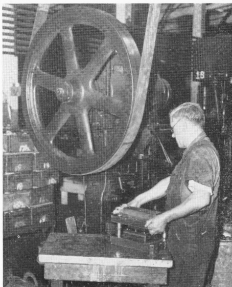
Once completed and tested, tool-setters like Aniello DiSantis, Blanking, can insert the tools which will produce new products.
